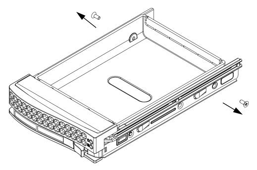
2 Slide the hard drive into the tray with the printed circuit board side facing down.
